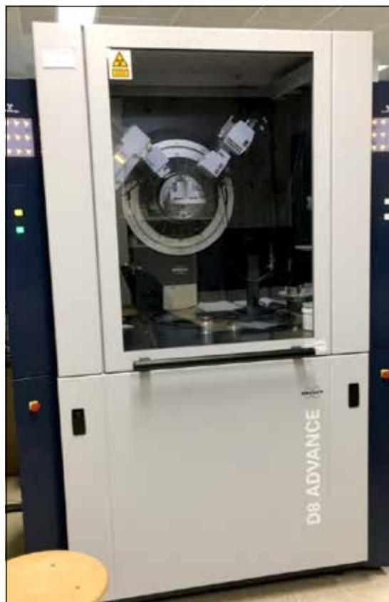
**Gambar 5.** *D8 Advanced Bruker Diffractometer*
